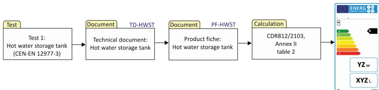
**Figure 1- Procedure for hot water storage tanks. The 'blue' codes are referring to one of the following tables and worksheets in the accompanying example workbooks.**
